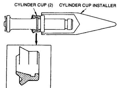
Installing the cylinder cup
