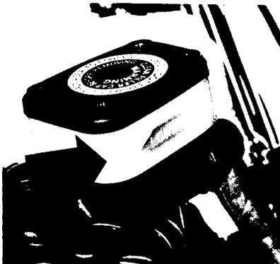
Front master cylinder brake fluid level line
