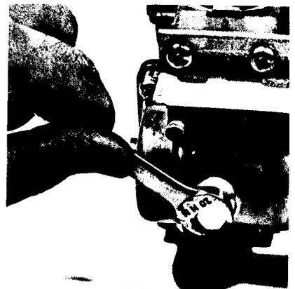
Removing the drain plug
