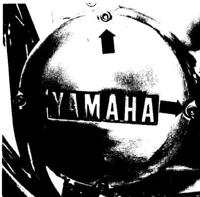
Alternator rotor cover allen bolts
