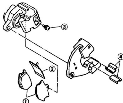
Caliper pad components: 1, pads; 2, pad spring; 3, screw; 4, retainers
