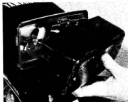
11.1a Stop/tail lamp lens is held by two screws as are ...
