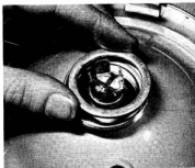
9.2b Note the special backing washers
