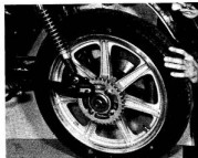
13.6 Tilt rear wheel and remove from the fork
