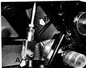
18.2 A = Pedal height bolt, B = Push rod adjuster nuts
