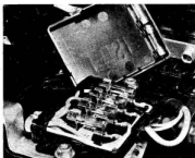
8.1 Spare fuses as contained in the fuse box lid
