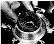
11.1b Oil seals may be prised out or drifted out with bearing
