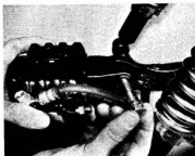
14.1a Rear disc caliper bolt has flat milled for location
