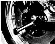
13.5b ... the rear wheel spindle to be withdrawn
