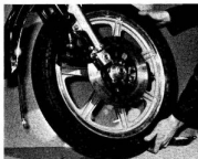
4.3b ... the front wheel to be lowered between the forks
