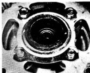
18.2b To separate sprocket from pins remove nuts
