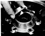
11.1a Remove spacers before drifting out bearings
