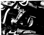
5.1 Voltage regulator is mounted below fuse box
