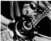
4.4b Wheel spindle clamp must be fitted with arrowmark forwards
