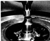
11.4b Drive in bearings using suitable tubular drift
