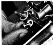
5.10c Pilot jet is enclosed by brass plug
