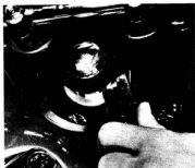
7.4 Adjust the steering head bearing using a 'C' spanner
