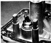
5.4c ... removal of the float needle
