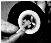
5.12e withdrawal of the needle seat and ...
