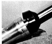
4.3b Prise off the dust excluder and withdraw ...
