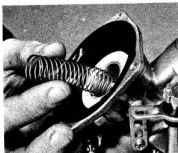
5.12b lift out the piston spring followed by ...
