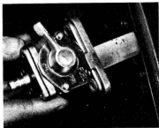
3.1 Withdraw the tap to gain access to the filter
