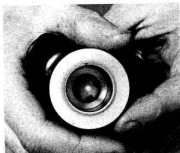
5.12d Remove the circlip to allow ...
