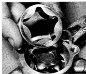
11.8 Fit outer rotor with punch marked face inwards
