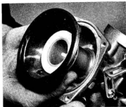
5.12c the piston/diaphragm unit
