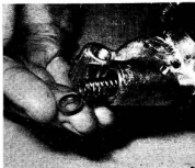
11.4b ... removal of the oil pressure release spring and ...
