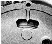
5.1b ... index pointer on casing allow ease of ignition timing
