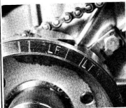
5.1a Timing marks on alternator rotor together with ...
