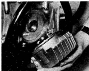
12.1b ... a hollow bolt containing the by-pass valve
