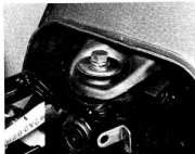
2.1 Petrol tank is retained at the rear by a single bolt
