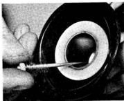
5.12f ... the piston needle, clip and spring
