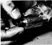
11.4c ... the pressure release valve plunger
