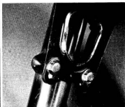
2.5a The mudguard is held by two bolts on each side
