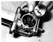
3.4b Lift out lever to gain access to seal and 'O' ring
