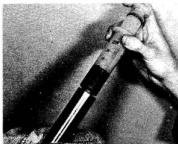
7.2 Refill each fork leg with the correct quantity of damping fluid
