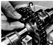
43.2 Insert and tighten sprocket retaining bolts
