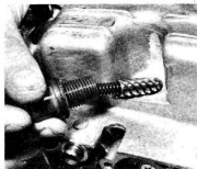
32.2 Replace the desert housing bolt, plunger and spring
