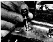
44.3b Note aluminium washers on two left-hand bolts
