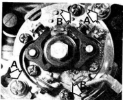
A = LH cylinder timing adjustment screws; B = RH cylinder screws
