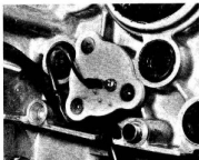
9.2b ... neutral indicator switch lead
