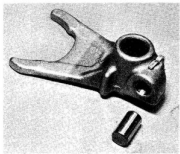
32.3a Fit the guide pins to the selector forks
