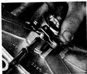
4.11 Detach clutch cable at operating mechanism
