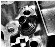
42.1a Fit the spring seat before fitting the new oil seal
