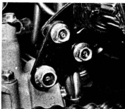
4.14d Detach upper bolt and also mounting plates
