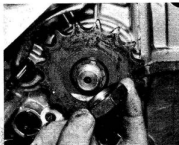
47.6a Replace the sprocket nut with relieved face inwards
