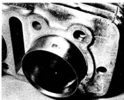
41.5c Check that cylinder 'O' rings are correctly positioned
