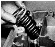
42.1c Install the spring with close wound pitch downward
