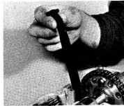
43.3a Refit the chain guide and ...
