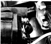
4.7 Detach starter lead at solenoid upper terminal
