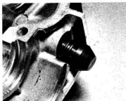
26.2a Left-hand rocker pins are held by rubber plugs
