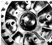
37.3d Install the clutch plates alternately and ...
