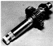
30.1a Check the condition of the kickstart clip
