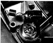
47.7a Check that the steel ball is fitted to the clutch
