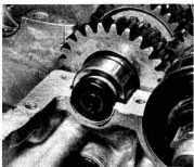
33.3 Install the clutch pushrod seal in end of the mainshaft
