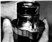
47.5b Split collars should be fitted as shown
