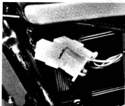
4.8a Main alternator leads connected by block connectors
