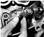
36.2a Place the pivot bush on the change arm stub and ....
