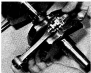
19.5a Separate the big-end bearing caps from connecting rods
