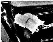
47.3 Alternator connectors cannot be incorrectly reconnected
