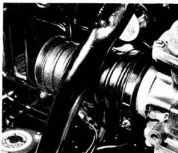
4.5a Pull air hose unit from carburetors and ...
