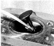
42.1b Lubricate the valve stem and guide thoroughly
