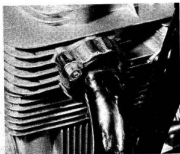
4.9b ... free the exhaust pipe flanges
