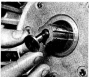
37.2d ... the clutch thrust piece
