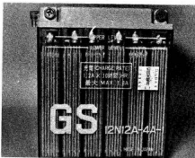
Electrolyte levels are clearly marked on battery
