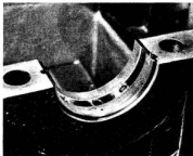
19.3a Check bearing shells for scoring or wear
