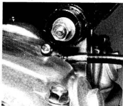
4.6 Tachometer cable is held by a single screw
