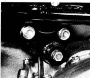
4.14a Detach the head steady, held by three bolts
