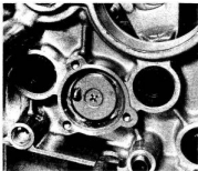
32.3e Drift both rod blind grommets into place
