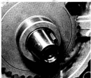
39.2a Fit the Woodruff key in the crankshaft and ...
